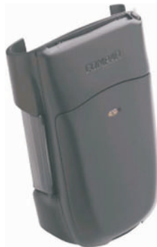
FIGURE 14-4 The iSwipe magnetic Card Reader allows your iPAQ to scan in Credit Cards.
